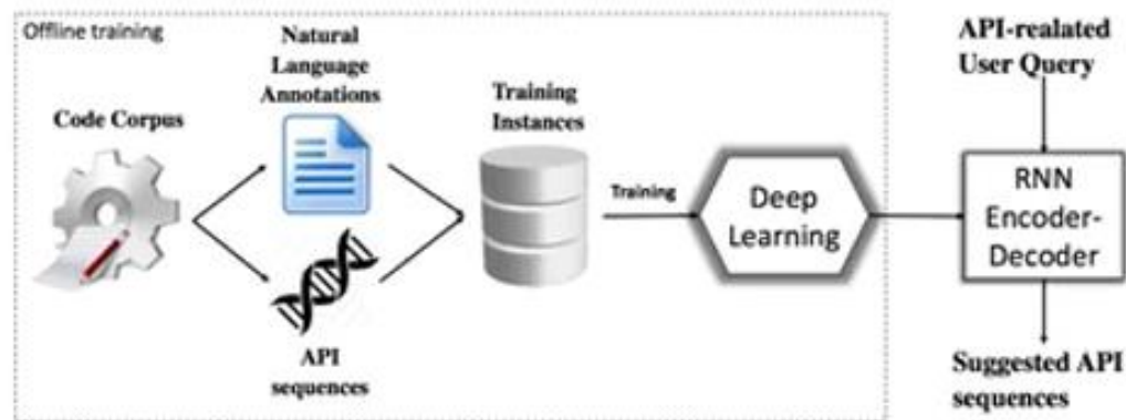
Figure 3: The Overall Workflow of DEEPAPI
